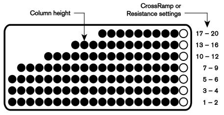
Figure 5: Parts of the program profile
